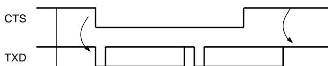
Figure 30-19. Transmitter Behavior when Operating with Hardware Handshaking
